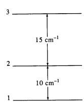
For the energy-level diagram above, what is the wave number of the transition from level 1 to level 3? (Wave number,  $\tilde{\nu}$ , is the reciprocal of
