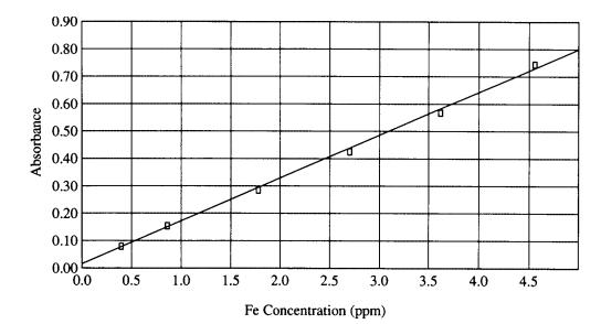
A working curve for the analysis of standard solutions of iron using atomic absorption spectrophotometry is shown above. The curve is most likely used to determine the
